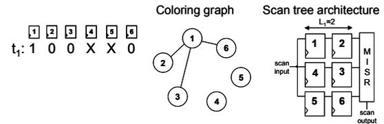
Figure 2. Scan tree generation from a test pattern
