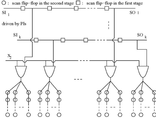
Fig. 3. Improved two-stage scan architecture.
