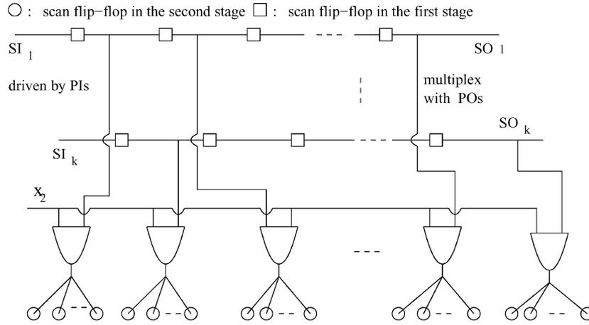
Fig. 1. Two-stage scan architecture.
