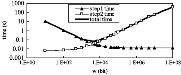
Fig. 11. Test time as a function of group size (at low error probability).
