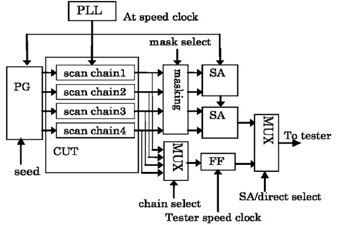
Fig. 7. BIST architecture for two-phase error identification.
