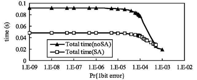
Fig. 14. Test time with and without signature analyzers.
