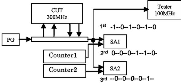
Fig. 6. Diagnosis with error detector signature analyzers.
