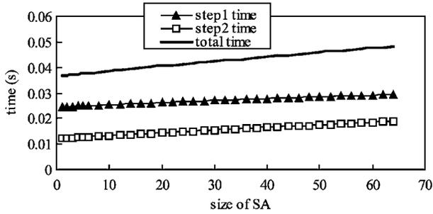
Fig. 15. Test time as a function of size of signature analyzers.
