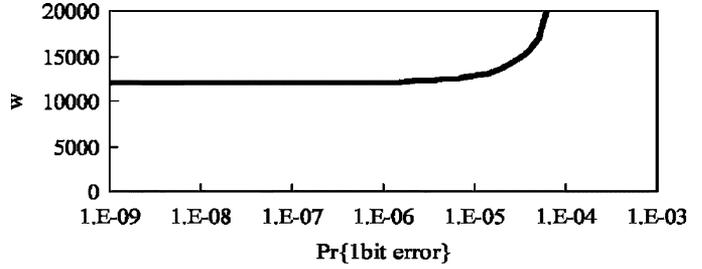
Fig. 13. Optimized group size as a function of the error probability (using signature analyzer in Step 2).
