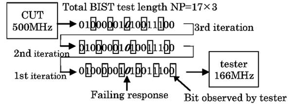
Fig. 3. Multiple iteration observation (successful).
