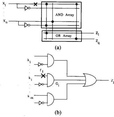
Fig. 1. Equivalent AND-OR circuit of PLA. (a) PLA. (b) Equivalent AND-OR.
