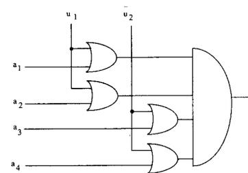
Fig. 7. Masking of AND gate.
