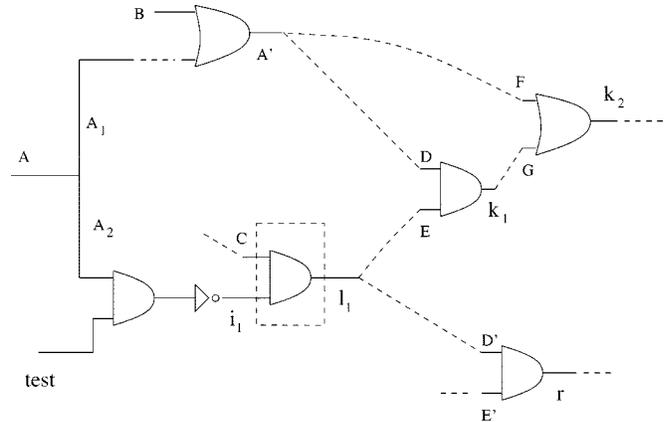
Fig. 2. Avoidance of conflicts generated by fault effect propagation.
