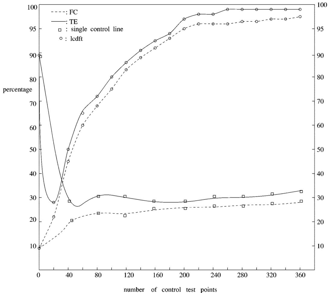
Fig. 5. Testability improvement for s13207.1 with various number of test points.
