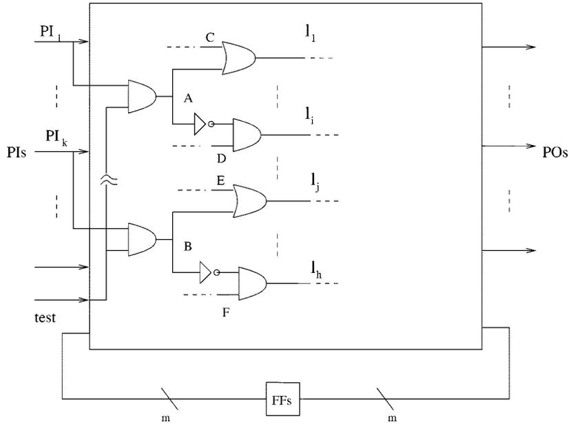
Fig. 1. Low-overhead nonscan DFT.
